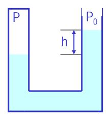
One can measure the pressure using an open-tube manometer, where one end is connected to the system with unknown pressure P and the other open to air with pressure  $P_0$ .
