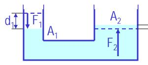
A<sub>2</sub> Since the pressure change caused by the the force F<sub>1</sub> applied onto the area A<sub>1</sub> is  $P = \frac{F_1}{A_1} = \frac{F_2}{A_2}$ transmitted to the  $F_2$  on an area  $A_2$ .  $F_2 = \frac{A_2}{A_1} F_1$  In other words, the force gets multiplied by the ratio of the areas  $A_2/A_1$  and is
