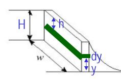
Since the water pressure varies as a function of depth, we will have to do some calculus to figure out the total force.
