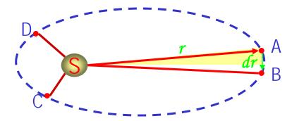
Since the gravitational force acting on the planet is always toward radial direction, it is a *central force* Therefore the torque acting on the planet by this force is always 0.
