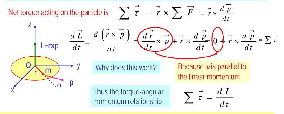
The net torque acting on a particle is the same as the time rate change of its angular momentum
