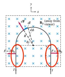
As in the previous example, the forces on the straight sections of the wire is equal and in opposite direction. Thus they cancel. What do we use to figure out the net force on the semicircle?  $d\vec{F} = Id\vec{l} \times \vec{B}$ We divide the semicircle into infinitesimal straight sections.  $dl = Rd\phi$
