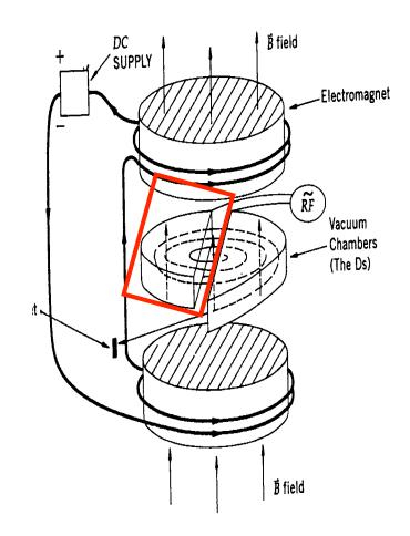
$$T_{\text{max}} = \frac{1}{2} m v_{\text{max}}^2 = \frac{1}{2} m \varpi^2 R^2 = \frac{(qBR)^2}{mc^2}$$
