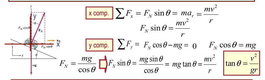
(b) What is this angle for an expressway off-ramp curve of radius 50m at a design speed of 50km/h?
