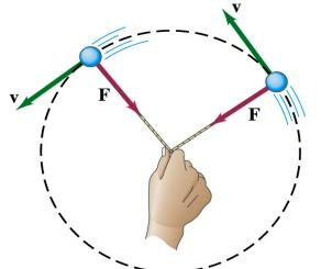
The <u>centripetal</u> \* acceleration is always perpendicular to the velocity vector, v, and points to the center of the axis (radial direction) in a uniform circular motion.
