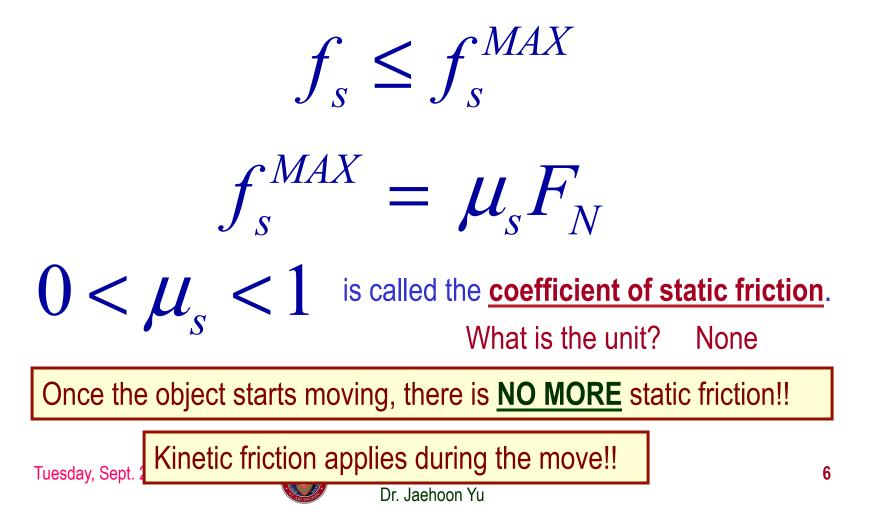
Note that the magnitude of the frictional force does not depend on the contact area of the surfaces.
