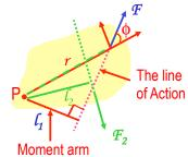
Consider an object pivoting about the point P by the force  $\mathcal{F}$  being exerted at a distance r from P. The line that extends out of the tail of the force vector is called the line of action.
