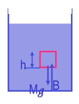
Let's consider a cube whose height **h** and cross sectional area **A** is filled with fluid and in its equilibrium so that its weight **Mg** is balanced by the buoyant force **B**.
