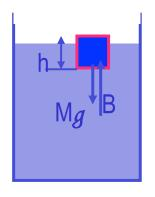
Let's consider an object of mass M, with density  $\rho_0$ , is in static equilibrium floating on the surface of the fluid with density  $\rho_f$ , and the volume submerged in the fluid is  $V_f$
