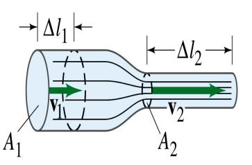
$$\frac{\Delta m_1}{\Delta t} = \frac{\rho_1 \Delta V_1}{\Delta t} = \frac{\rho_1 A_1 \Delta l_1}{\Delta t} = \rho_1 A_1 v_1$$
