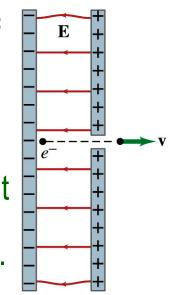
The magnitude of the force on the electron is F=qE and is directed to the right. The equation to solve this problem is
