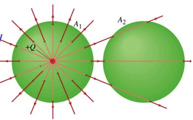
The surface A<sub>1</sub> encloses the charge +Q, so from Gauss' law we obtain the total net flux
