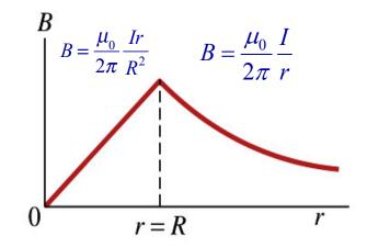
**Coaxial cable.** A coaxial cable is a single wire surrounded by a cylindrical metallic braid, as shown in the figure. The two conductors are separated by an insulator. The central wire carries current to the other end of the cable, and the outer braid carries the return current and is usually considered ground. Describe the magnetic field (a) in the space between the conductors and (b) outside the cable.
