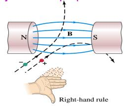
**Magnetic force on a proton.** A proton having a speed of 5x10<sup>6</sup>m/s in a magnetic field feels a force of F=8.0x10<sup>-14</sup>N toward West when it moves vertically upward. When moving horizontally in a northerly direction, it feels zero force. What is the magnitude and the direction of the magnetic field in this region?
