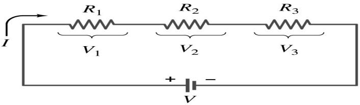
• What is the potential energy loss when charge q passes through resistors R<sub>1</sub>, R<sub>2</sub> and R<sub>3</sub>
