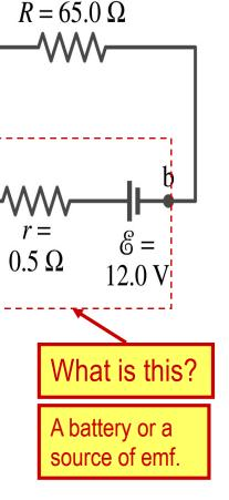
(b) The terminal voltage  $V_{ab}$  is  $V_{ab} = \mathcal{E} - Ir = 12.0V - 0.183A \cdot 0.5\Omega = 11.9V$
