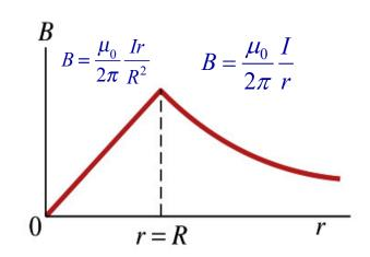
Coaxial cable. A coaxial cable is a single wire surrounded by a cylindrical metallic braid, as shown in the figure. The two conductors are separated by an insulator. The central wire carries current to the other end of the cable, and the outer braid carries the return current and is usually considered ground. Describe the magnetic field (a) in the space between the conductors and (b) outside the cable.
