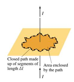
– The sum of all the products of the length of each segment and the component of B parallel to that segment is equal to  $\mu_0$  times the net current  $I_{\text{encl}}$  that passes through the surface enclosed by the path
