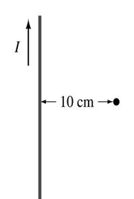
Using the formula for the magnetic field near a straight wire
