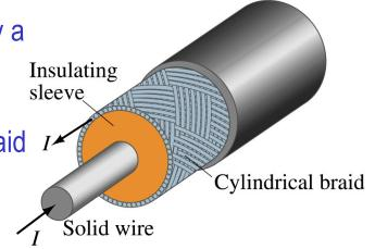
(a) The magnetic field between the conductors is the same (a) The magnetic field between the conductors is the same as the long, straight wire case since the current in the outer  $B=\frac{\mu_0}{2\pi}\frac{I}{r}$ conductor does not impact the enclosed current.
