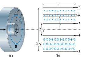
(a) The total flux through  $\ell$  of the cable is  $\Phi_B = \int Bl \, dr = \frac{\mu_0 Il}{2\pi} \int_{r_1}^{r_2} \frac{dr}{r} = \frac{\mu_0 Il}{2\pi} \ln \frac{r_2}{r_1}$
