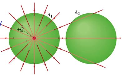
The surface A<sub>1</sub> encloses the charge +Q, so from Gauss' law we obtain the total net flux
