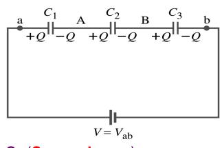
**Equivalent Capacitor:** Determine the capacitance of a single capacitor that will have the same effect as the combination shown in the figure. Take  $C_1=C_2=C_3=C$ .
