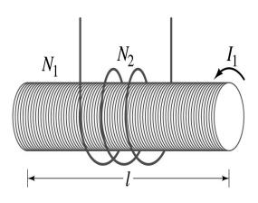
First we need to determine the flux produced by the solenoid. What is the magnetic field inside the solenoid?  $B = \frac{\mu_0 N_1 I_1}{r}$
