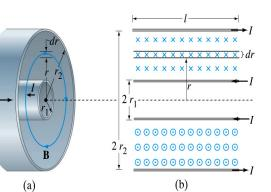
(a) The total flux through  $\ell$  of the cable is  $\Phi_B = \int Bl \, dr = \frac{\mu_0 Il}{2\pi} \int_{r_1}^{r_2} \frac{dr}{r} = \frac{\mu_0 Il}{2\pi} \ln \frac{r_2}{r_1}$
