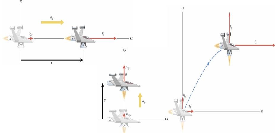
Imagine you add the two 1 dimensional motions on the left. It would make up a one 2 dimensional motion on the right.
