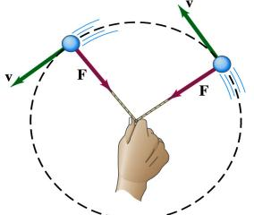
The <u>centripetal</u> \* acceleration is always perpendicular to the velocity vector, v, and points to the center of the axis (radial direction) in a uniform circular motion.
