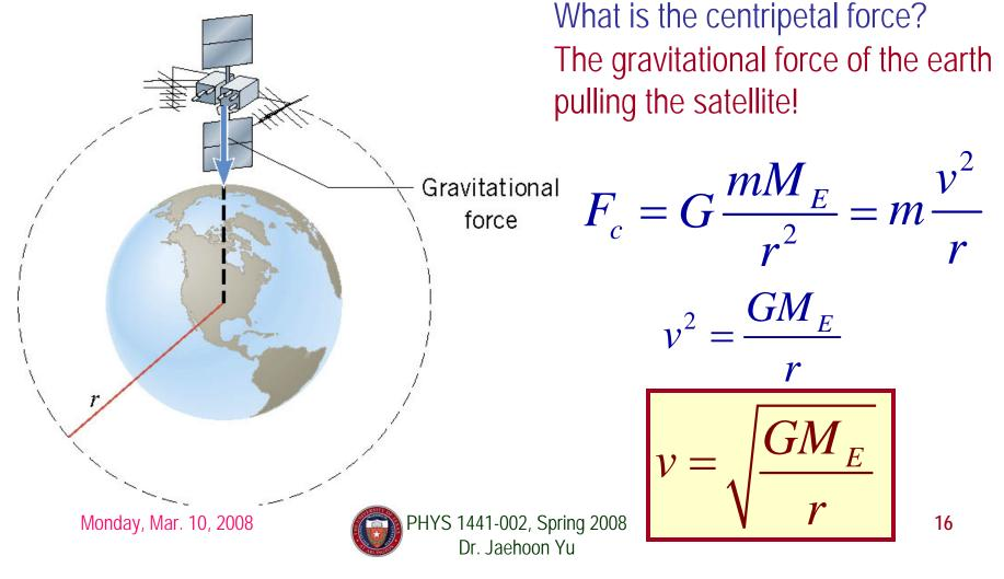
Ex. 9 Orbital Speed of the Hubble Space Telescope Determine the speed of the Hubble Space Telescope orbiting at a height of 598 km above the earth's surface.
