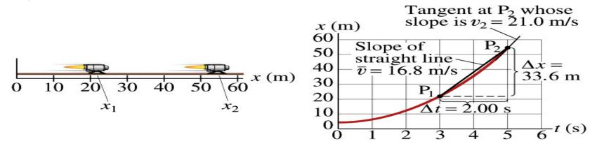
(a) Determine the displacement of the engine during the interval from  $t_1$ =3.00s to  $t_2$ =5.00s.  $x_1 = x_{t_1=3.00} = 2.10 \times (3.00)^2 + 2.80 = 21.7m$   $x_2 = x_{t_2=5.00} = 2.10 \times (5.00)^2 + 2.80 = 55.3m$
