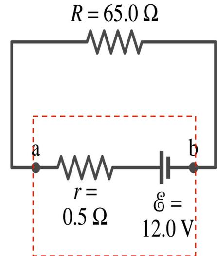
(a) Since  $V_{ab} = \mathcal{E} - Ir$  We obtain  $V_{ab} = IR = \mathcal{E} - Ir$
