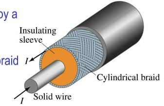
(a) The magnetic field between the conductors is the same as the long, straight wire case since the current in the outer conductor does not impact the enclosed current.
