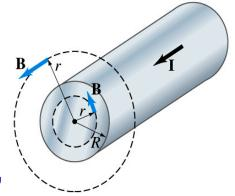
Since the wire is long, straight and symmetric, the field should be the same at any point the same distance from the center of the wire.
