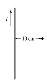
Using the formula for the magnetic field near a straight wire
