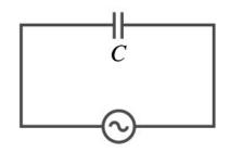
The peak voltage is  $V_0 = \sqrt{2}V_{rms} = 120V \cdot \sqrt{2} = 170V$
