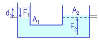
$\begin{array}{c|c} A_2 \\ \hline \\ F_2 \end{array} = \begin{array}{c} A_2 \\ d_2 \end{array} \begin{array}{c} \text{Since the pressure change caused by the} \\ \text{the force } F_1 \text{ applied onto the area } A_1 \text{ is} \end{array} P = \frac{F_1}{A_1} = \frac{F_2}{A_2} \end{array}$ transmitted to the  $F_2$  on an area  $A_2$ .  $F_2 = \frac{A_2}{A_1} F_1$  In other words, the force gets multiplied by the ratio of the areas A<sub>2</sub>/A<sub>1</sub> and is
