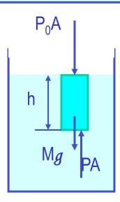
It seems that the pressure has a lot to do with the total mass of the fluid above the object that puts weight on the object.
