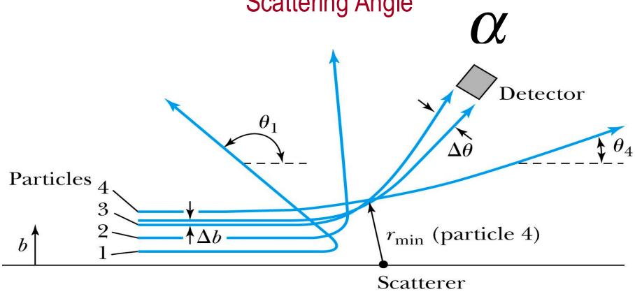
The relationship between the impact parameter b and scattering angle  $\theta$ : Particles with small impact parameters approach the nucleus most closely  $(r_{min})$  and scatter to the largest angles. Particles within a certain range of impact parameters b will be scattered within the window  $\Delta\theta$ .
