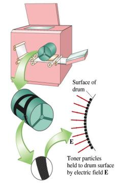
The electric force must be the same as twice the gravitational force on the toner particle.
