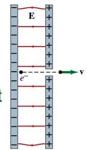
The magnitude of the force on the electron is F=qE and is directed to the right. The equation to solve this problem is
