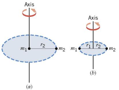
Which case is easier to spin?Case (b)Why? Because the moment of inertia is smaller
