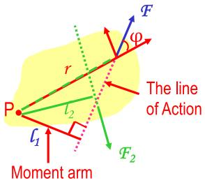
Consider an object pivoting about the point P by the force  $\boldsymbol{\mathcal{F}}$  being exerted at a distance r from P.
