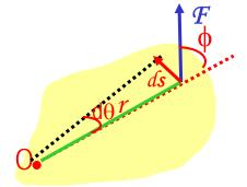
Let's consider a motion of a rigid body with a single external force  $\mathcal{F}$  exerting on the point P, moving the object by ds. The work done by the force  $\mathcal{F}$  as the object rotates through the infinitesimal distance ds=rd $\theta$  is
