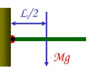
The only force generating torque is the gravitational force  $\mathcal{M}g$
