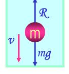
$\sum \vec{F} = \vec{F}_g + \vec{R} = m\vec{a} \quad \sum F_x = 0 \quad \text{In other words}$  $\sum F_y = mg - bv = ma = m\frac{dv}{dt} \quad \frac{dv}{dt} = g - \frac{b}{m}v \quad \frac{dv}{dt} = g - \frac{b}{m}v = g, \text{ when } v = 0$
