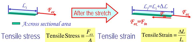
$$Y \equiv \frac{\text{Tensile Stress}}{\text{Tensile Strain}} = \frac{F_{ex}}{\frac{A}{\Delta L}}$$
