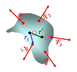
If an object is at its translational static equilibrium, and if the net torque acting on the object is 0 about one axis, the net torque must be 0 about any arbitrary axis.
