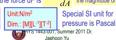
Note that pressure is a scalar quantity because it's the magnitude of the force on a surface area A.
