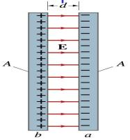
**Capacitor calculations:** (a) Calculate the capacitance of a capacitor whose plates are 20cmx3.0cm and are separated by a 1.0mm air gap. (b) What is the charge on each plate if the capacitor is connected to a 12-V battery? (c) What is the electric field between the plates? (d) Estimate the area of the plates needed to achieve a capacitance of 1F, given the same air gap.
