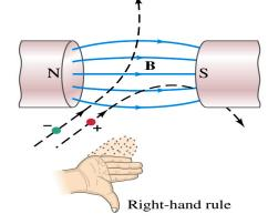
**Magnetic force on a proton.** A proton having a speed of 5x10<sup>6</sup>m/s in a magnetic field feels a force of F=8.0x10<sup>-14</sup>N toward the west when it moves vertically upward. When moving horizontally in a northerly direction, it feels zero force. What is the magnitude and direction of the magnetic field in this region?
