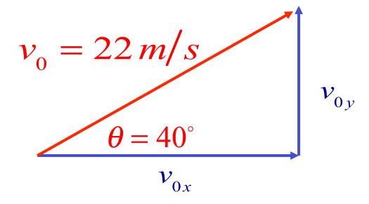
$$v_{0x} = v_o \cos \theta = (22 \text{ m/s}) \cos 40^\circ = 17 \text{ m/s}$$
