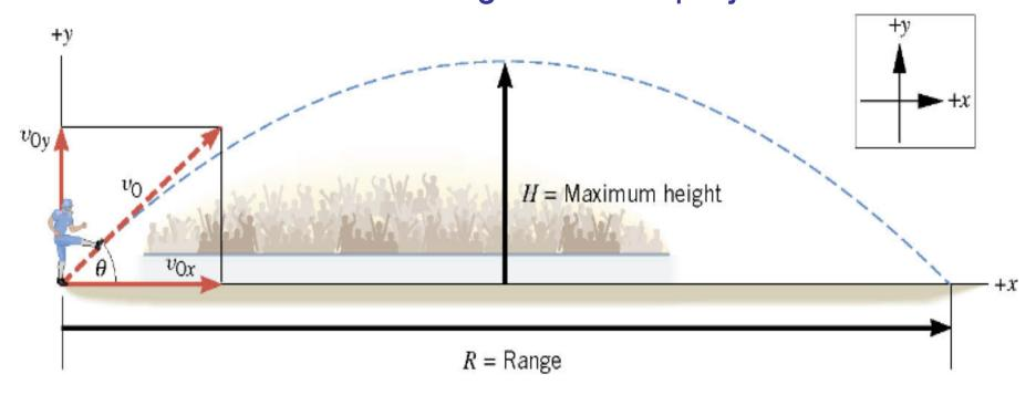
$$x = v_{ox}t + \frac{1}{2}a_xt^2 = v_{ox}t = (17 \text{ m/s})(2.9 \text{ s}) = +49 \text{ m}$$
