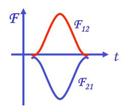
Assuming no external forces, the force exerted on particle 1 by particle 2,  $\mathcal{F}_{21}$ , changes the momentum of particle 1 by
