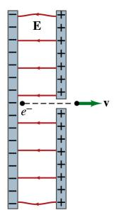
The magnitude of the force on the electron is F=qE and is directed to the right. The equation to solve this problem is
