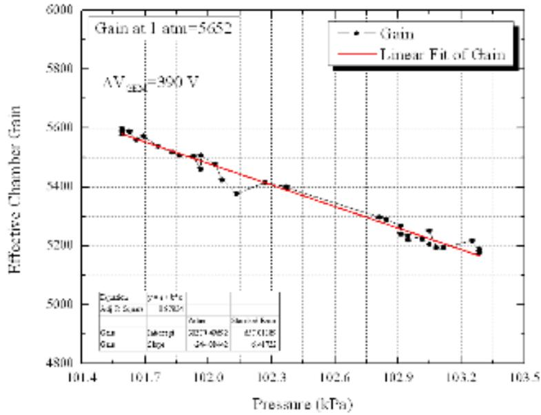
**FIGURE 8.** The Gain versus pressure dependence graph
