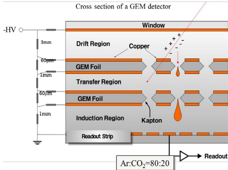
FIGURE 1. GEM detector cross section
