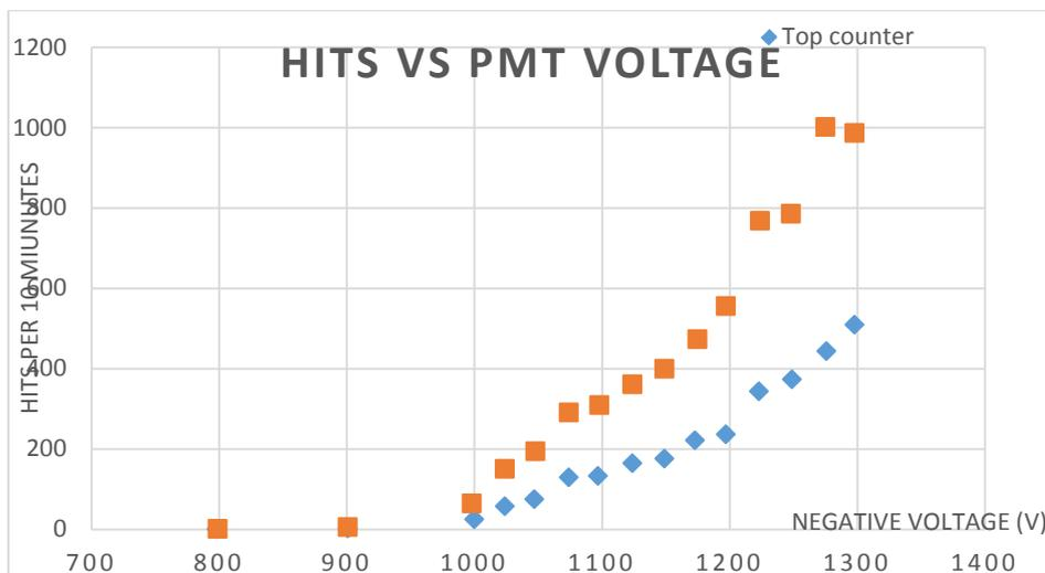
**FIGURE 7.** Number of hit count vs PMT operating voltage
