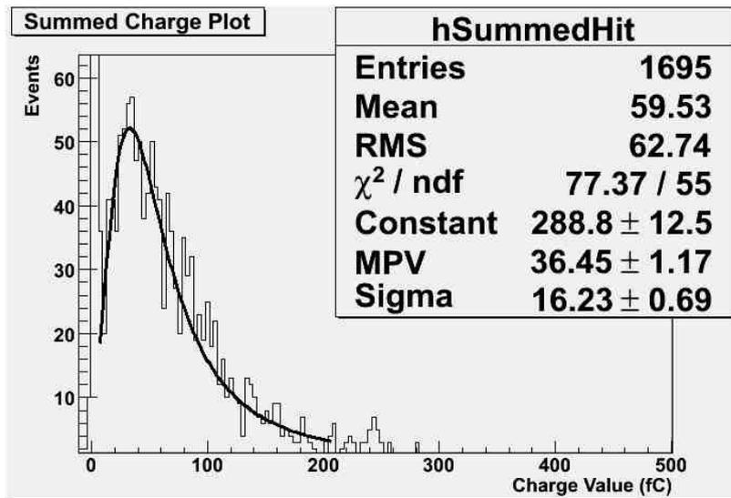
**FIGURE 9.** A charge distribution of cosmic radiation created by the GEM detector coupled with the KPiX chip with a distinct landau fit.
