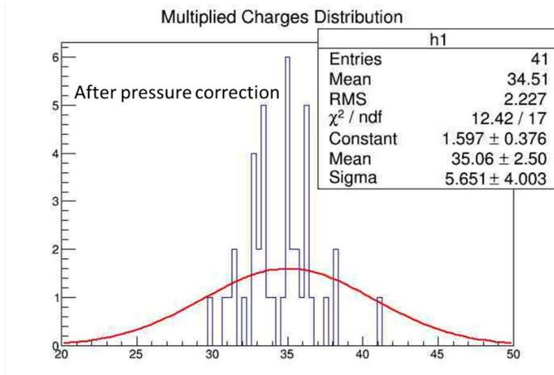
**FIGURE 12.** Multiplied charge distribution after pressure correction (Fit:Normal)
