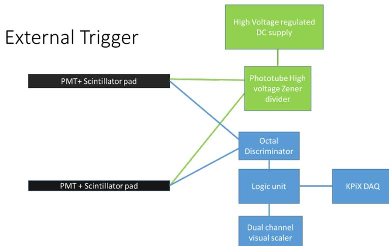
**FIGURE 4.** The external trigger layout. The Green block is the power supply block, while the blue blocks are the signal discriminator block.
