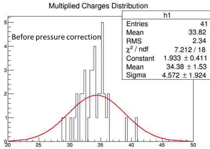
**FIGURE 11.** Multiplied charge distribution before pressure correction (Fit: Normal)
