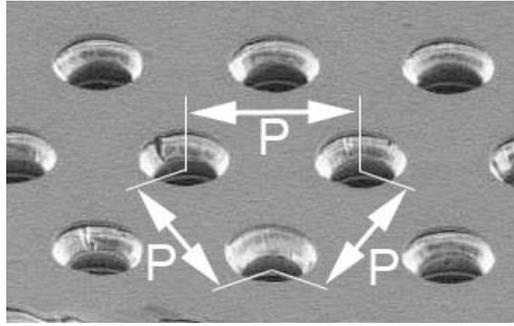
**FIGURE 3.** prototype 28cm x28cm GEM foil with a pitch of 180 micrometer.
