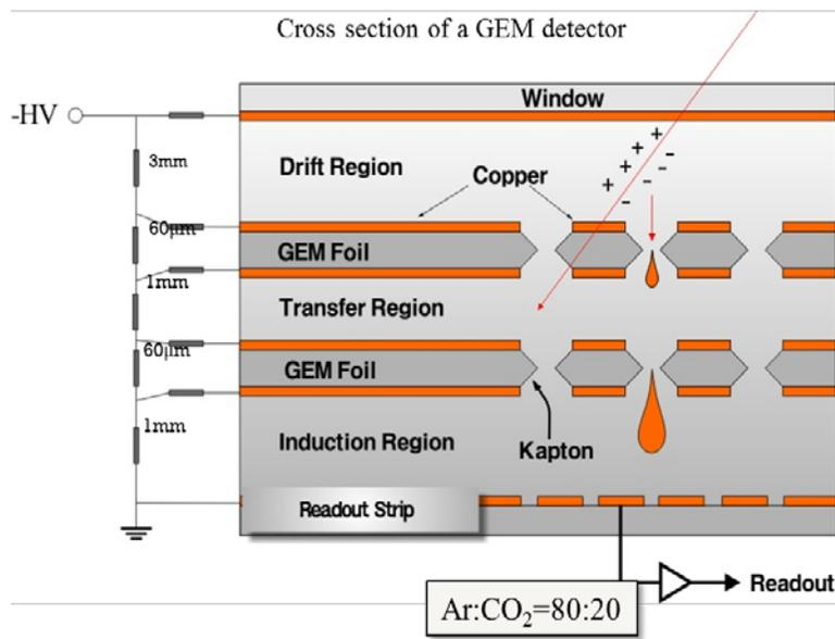
FIGURE 2. GEM detector cross section
