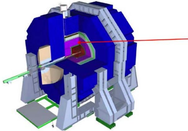
**FIGURE 1.** The SID detector of the ILC. The violet part is where the DHAL system is intended to be installed.
