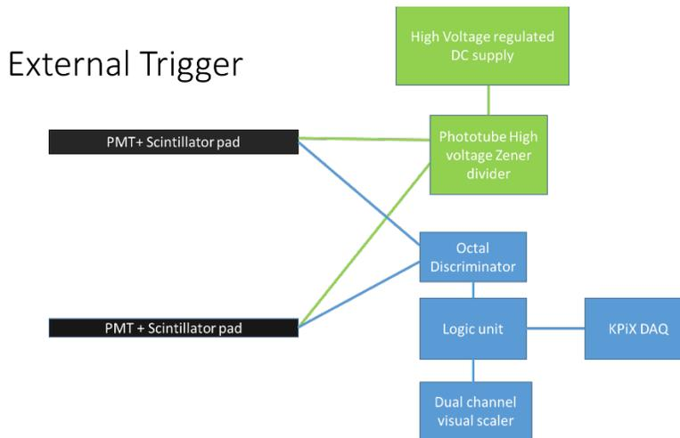
**FIGURE 6.** The external trigger layout. The Green block is the power supply block, while the blue blocks are the signal discriminator block.
