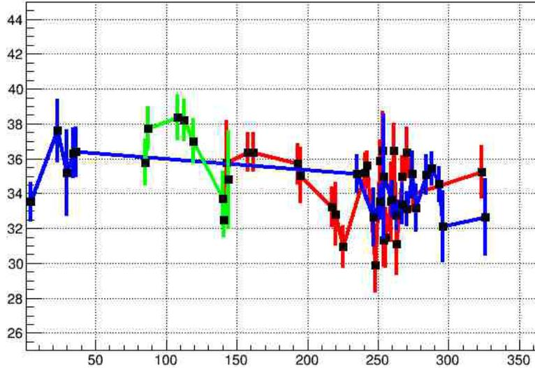
**FIGURE 9:** MPV of multiplied charge value distribution vs days of the year (Red: 2012, Blue: 2013, Green: 2014)
