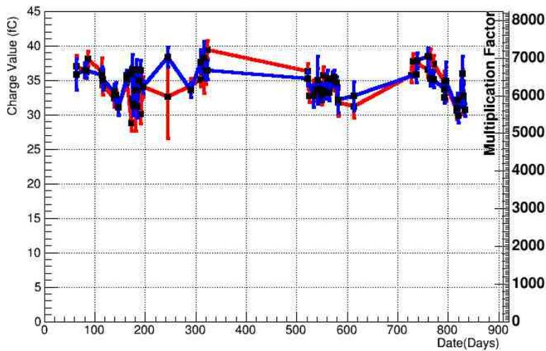
**FIGURE 8 :**MPV of multiplied charge distribution vs days (Red: Before pressure correction; Blue: After pressure correction)
