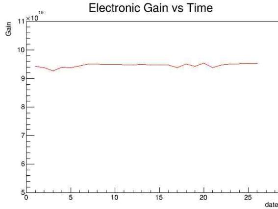
**FIGURE 14:** Electronic gain (ADC/fC) vs months (channel 0)
