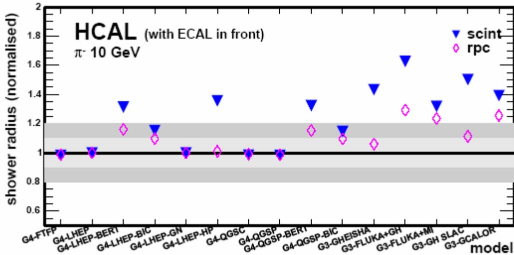
**Figure 1. Comparison of the shower radius in a hadronic calorimeter as predicted by fifteen different MC models of hadronic showers. Differences from a few % to as large as 60% between different models can be seen.**
