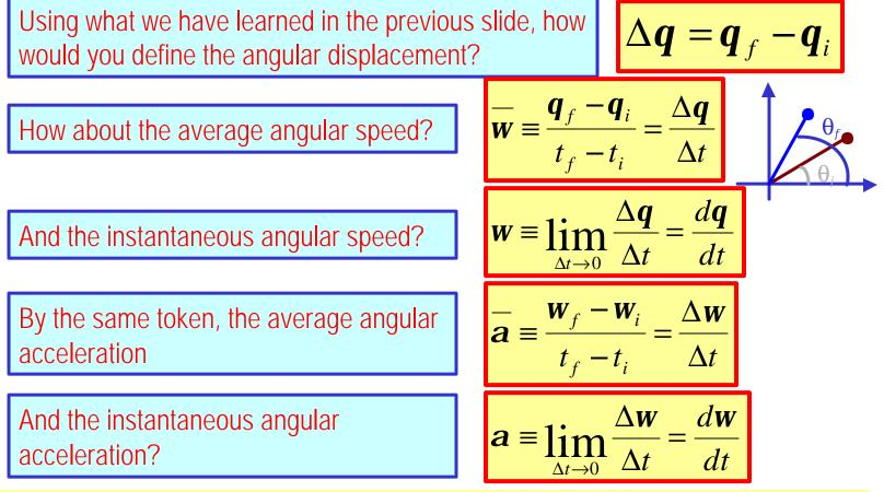
When rotating about a fixed axis, every particle on a rigid object rotates through the same angle and has the same angular speed and angular acceleration. Wednesday, Oct. 23, 2002 PHYS 1443-003, Fall 2002 Dr. Jaehoon Yu
