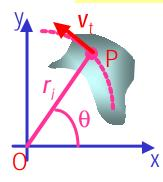
When a point rotates, it has both the linear and angular motion components in its motion.
