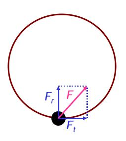
*The object has both tangential and radial accelerations.*
