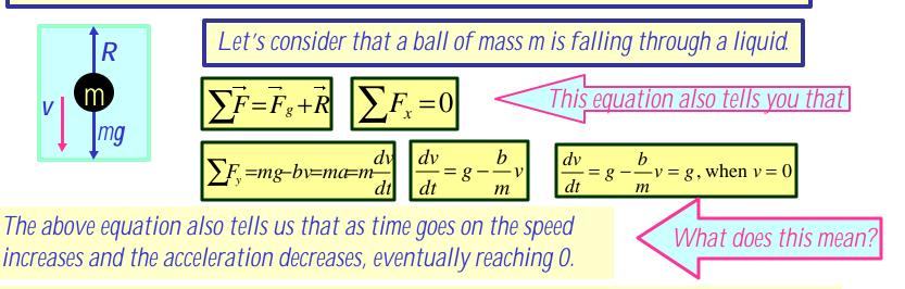
An object moving in a viscous medium will obtain speed to a certain speed (**terminal speed**) and then maintain the same speed without any more acceleration.
