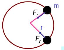
The centripetal acceleration is always perpendicular to velocity vector,  $\mathbf{v}$ , for uniform circular motion.
