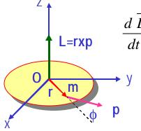
$$\frac{d\vec{L}}{dt} = \frac{d(\vec{r} \times \vec{p})}{dt} = \underbrace{\frac{d\vec{r}}{dt} \times \vec{p}}_{\text{th}} + \vec{r} \times \frac{d\vec{p}}{dt} = 0 + \vec{r} \times$$
