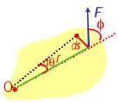
Let's consider a motion of a rigid body with a single external force **F** exerting on the point P, moving the object by **ds**. The work done by the force **F** as the object rotates through the infinitesimal distance  $ds=rd\theta$  is
