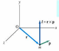
Let's consider a point-like object (particle) with mass m located at the vector location *r* and moving with linear velocity *v*
