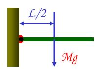
The only force generating torque is the gravitational force  $\mathcal{M}_{\boldsymbol{g}}$
