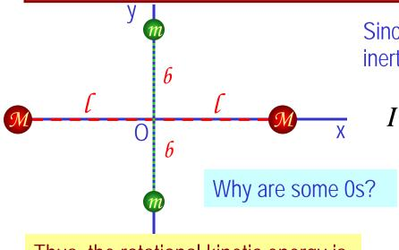
Since the rotation is about y axis, the moment of inertia about y axis,  $I_{y'}$  is
