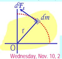
The torque due to tangential force  $\mathcal{F}_t$  is  $d\tau = dF_t r = (r^2 dm)\alpha$
