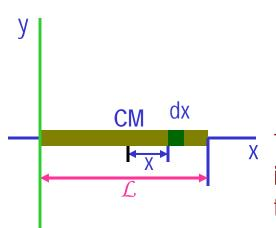
The line density of the rod is  $\lambda = \frac{M}{L}$  so the masslet is  $dm = \lambda dx = \frac{M}{L} dx$
