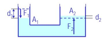
Since the pressure change caused by the the force  $F_1$  applied on to the area  $A_1$  is transmitted to the  $F_2$  on an area  $A_1$ . transmitted to the  $F_2$  on an area  $A_2$ .
