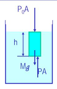
It seems that the pressure has a lot to do with the total mass of the fluid above the object that puts weight on the object.
