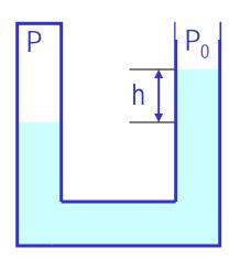
One can measure the pressure using an open-tube manometer, where one end is connected to the system with unknown pressure P and the other open to air with pressure  $P_0$ .
