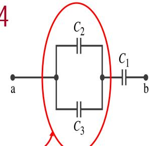
How? These are in parallel so the equivalent capacitance is:
