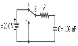
(a) Since the current reaches to 0.5 of its initial value in  $40\mu$ s, we can obtain  $I(t) = I_0 e^{-t/RC} \quad \text{For } 0.5I_0 = I_0 e^{-t/RC} \quad \text{Rearrange terms} - t/RC = \ln 0.5 = -\ln 2$ Solve for R  $R = t/(C \ln 2) = 40 \times 10^{-6}/(1.02 \times 10^{-6} \cdot \ln 2) = 56.6\Omega$ (b) The value of Q at t=0 is
