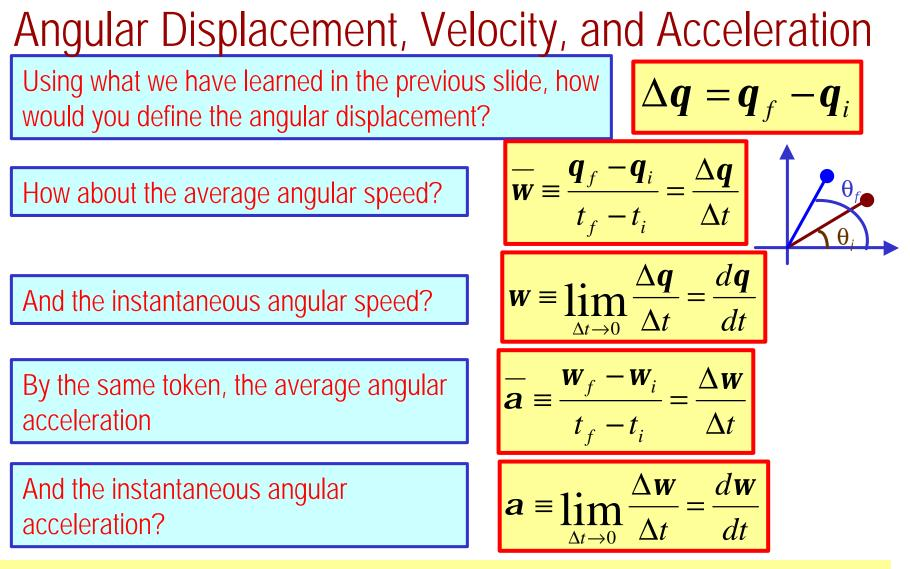
When rotating about a fixed axis, every particle on a rigid object rotates through the same angle and has the same angular speed and angular acceleration. Mar. 4, 2002 1443-501 Spring 2002 6
