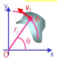
When a point rotates, it has both the linear and angular motion components in its motion. The
