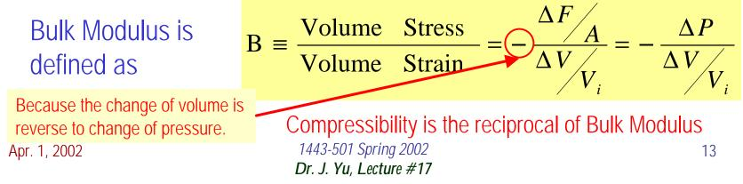
A solid brass sphere is initially under normal atmospheric pressure of  $1.0x10^5$ N/m<sup>2</sup>. The sphere is lowered into the ocean to a depth at which the pressures is  $2.0x10^7$ N/m<sup>2</sup>. The volume of the sphere in air is 0.5m<sup>3</sup>. By how much its volume change once the sphere is submerged?
