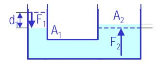
Since the pressure change caused by the =  $d_2$  the force  $F_1$  applied on to the area  $A_1$  is transmitted to the  $F_2$  on an area  $A_2$ .
