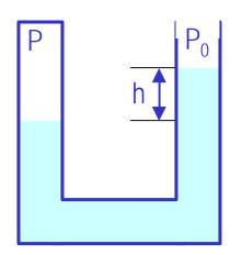
One can measure pressure using an open-tube manometer, where one end is connected to the system with unknown pressure P and the other open to air with pressure  $P_0$ .
