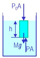
It seems that the pressure has a lot to do with the total mass of the fluid above the object that puts weight on the object.
