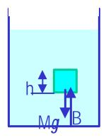
Let's consider a cube whose height is h and is filled with fluid and at its equilibrium. Then the weight Mg is balanced by the buoyant force B.
